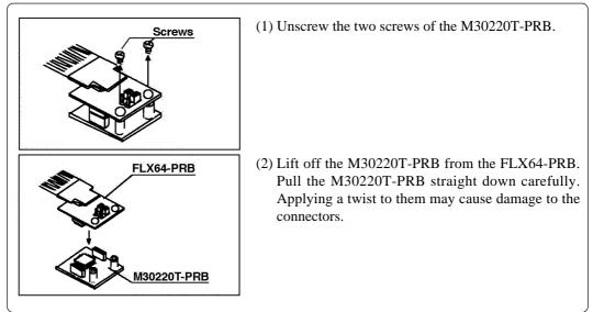
Figure 3.4 Removing the M30220T-PRB pod probe
